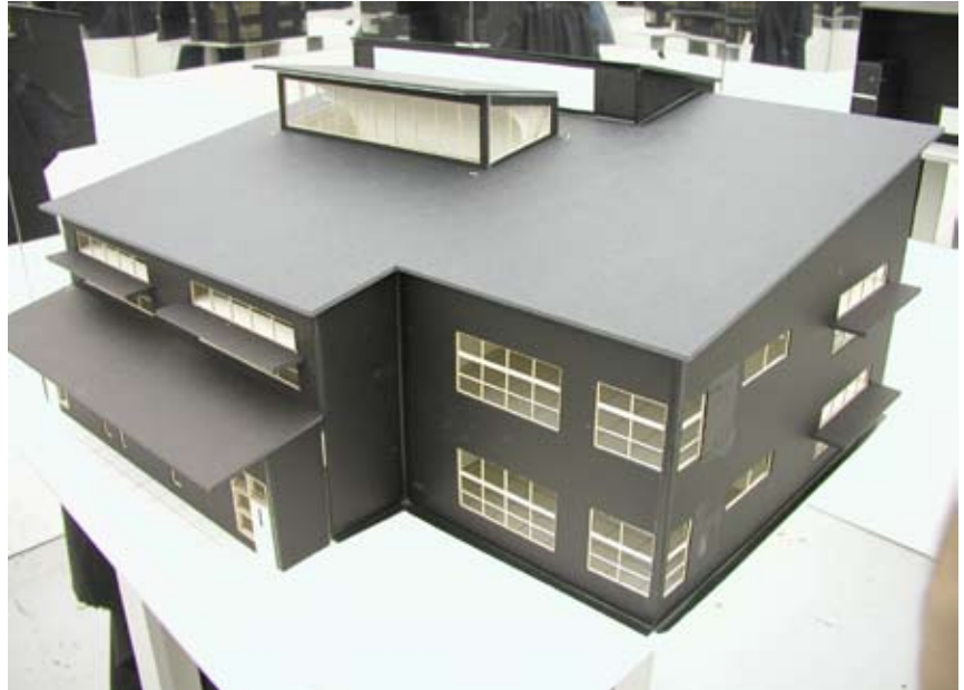
This heliodon model of Mt. View Elementary School was used by designers to formulate daylighting strategies. The physical models studied on a heliodon helped to define appropriate sun control for windows and placement of interior light shelves to let daylight reach into rooms.
