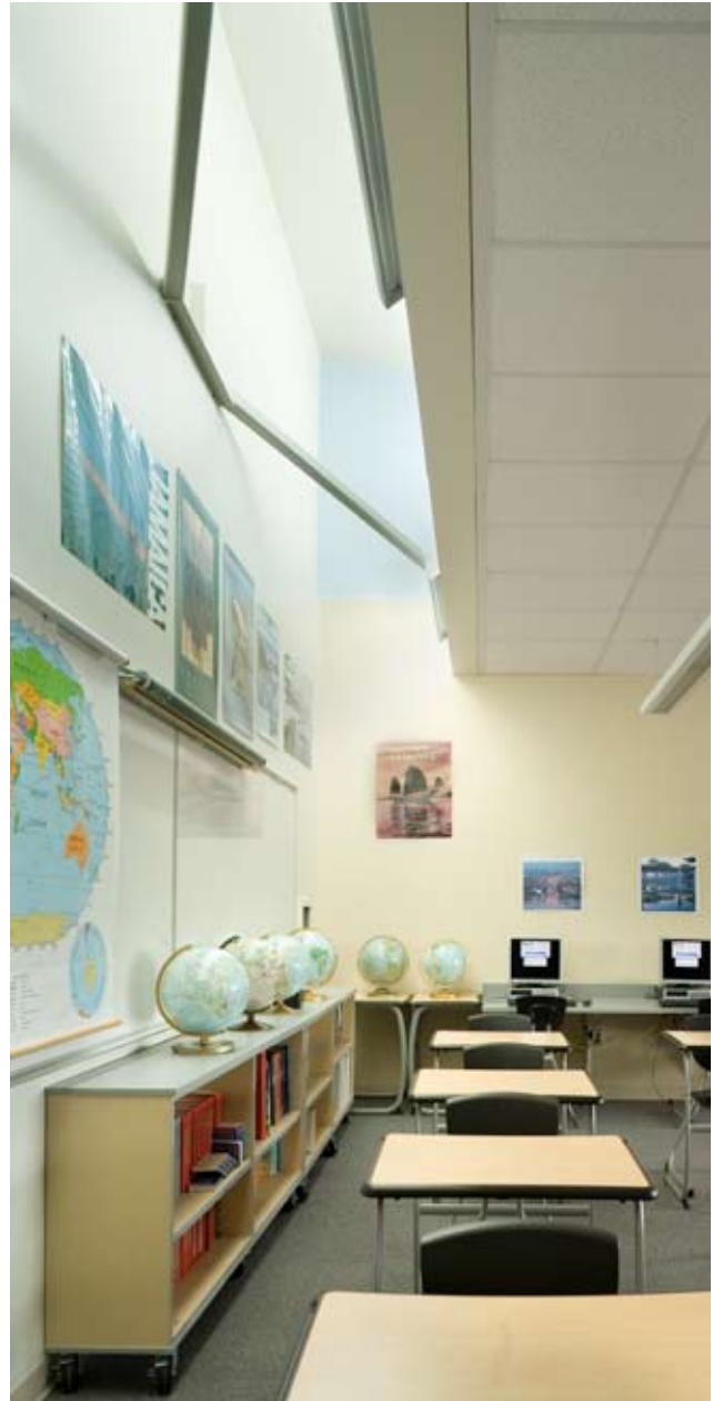
A classroom in the Wilson High School takes advantage of natural light by means of a lighting shelf. Models and calculations were used to predict the amount of light this approach would provide.
